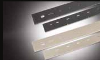
Rear squeegee rubber blades 33 SHORE (PARA) For maintenance cleaning of smooth floors. 40 SHORE (PARA) For stubborn dirt on floors with joints. POLYURETHANE For heavy duty cleaning on industrial floors, even with wide gaps.
