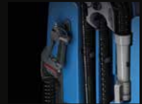
Sanitizing sprayer to sanitize the machine at the end of the shift (only available with the Disinfector kit)
